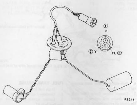
Fig. FE-10 Fuel tank gauge
