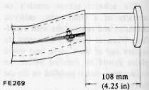
Fig. FE-16 Mounting position of exhaust front tube heat shield plate
