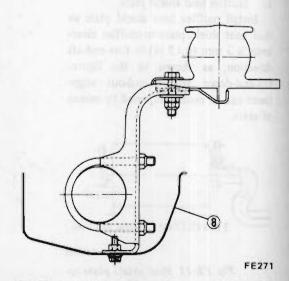
Fig. FE-18 Exhaust front tube mounting bracket
