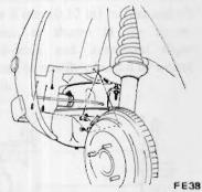
Fig. FE-8 Removing fuel filler hose protector
