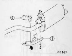
Fig. FE-14 Installing upper heat shield plate
