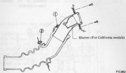
Fig. FE-9 Cross-sectional view of fuel hose
