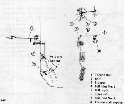
Fig. FE-4 Accelerator linkage setting
