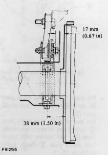
Fig. FE-12 Installing muffler front mounting
